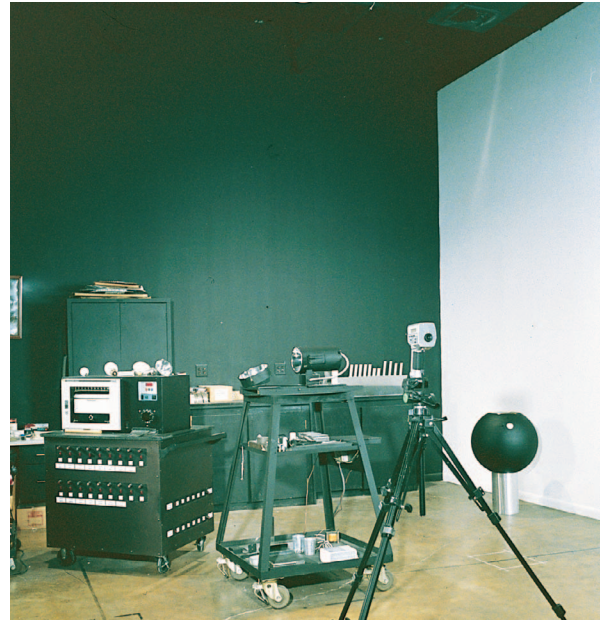
Kurt Versen's photometric laboratory showing set-up for Maximum Brightness Method testing.
